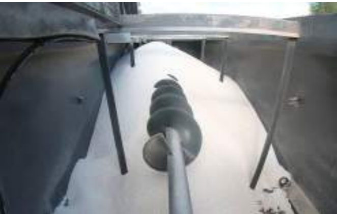
Trash wheel for optimal discharge of the fertiliser tank
