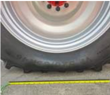
ATP Control – increased contact area at 1.0 bar tyre pressure
