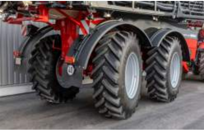
Active steering with a steering angle of up to 28° for maximum crop protection
