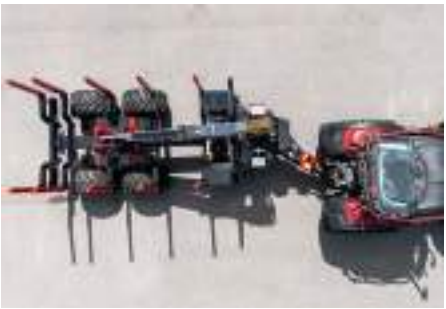
The forwarder can be laterally shifted by up to 104 cm with the drawbar
