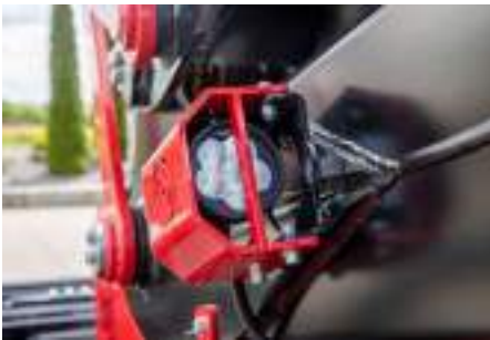
WorkLight: protected crane headlight as an option
