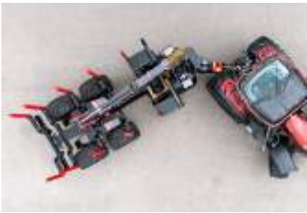
Utmost manoeuvrability due to large steering angle of the drawbar
