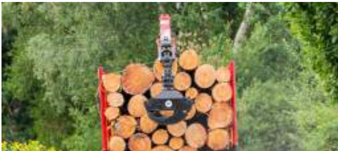
During road transport, the grapple is attached behind the vehicle
