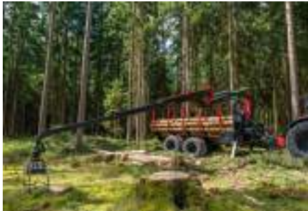
IB 9800.L10 with up to 10 m range and 2.2 t lifting power with an outreach of 4 m
