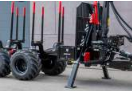
A-column support integrated into the front grid
