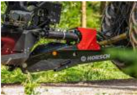
In the lowered position, the lateral skidding of the vehicle is prevented by the mechanical end stop of the cylinder.
