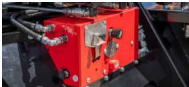
Brake load adjustment at the drawbar
